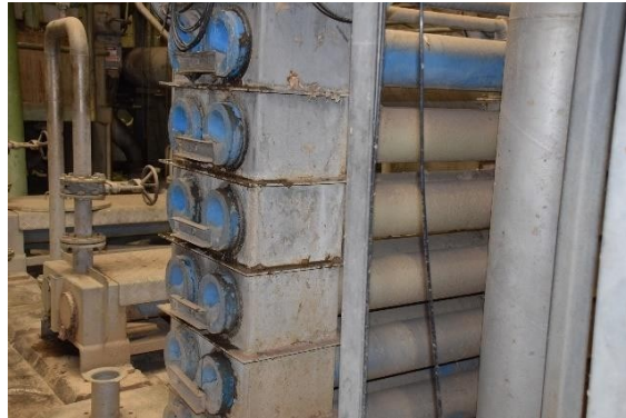
Two stage Light-weight cleaner system Voith Cyclean 1 st Stage: 14 cleaners installed 2 nd Stage: 2 cleaners installed
