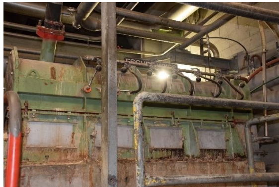
Stock Approach Rejectsorter (common with Topformer Approach flow) Escher-Wyss Model RS2B Speed: 1190 rpm Input Power: 55 kW @ 1480 rpm. 2.6mm holes, 44% open area
