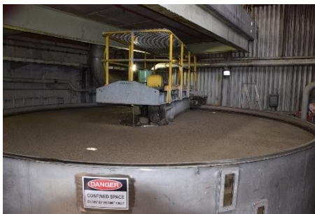
Purgomat PU66 Escher-Wyss 6600mm diameter
